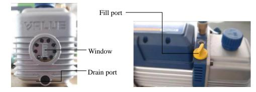
Note: the new vacuum pump oil cannot be filled too much into the vacuum pump otherwise it will spray out when working. C-4: Re-back the cover.
