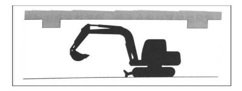
Please do not make the mini-excavator overload or overlength during hoisting. Over load can result in the overturn of the mini-excavator, thus resulting in serious injury to personnel or death.
