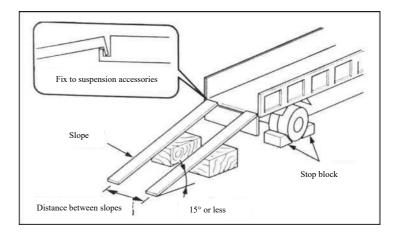
During loading and unloading, the mini-excavator may overturn or fall. Please take the following safety measures:
