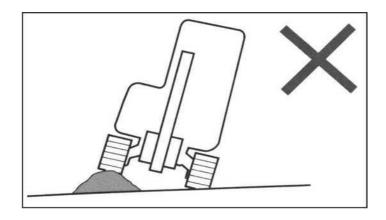
Do not operate the mini-excavator on an excessively steep slope where the mini-excavator cannot keep its stability (Maximum slope: 30°, lateral inclination: 10°); Please note that in fact, depending on the working conditions, the stability of the mini-excavator will be lower than the above value.
