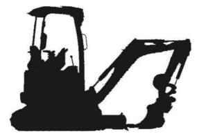
When the excavation operation is completed or the operation of the mini-excavator is stopped, the bucket of the mini-excavator should be lowered to the ground and the key should be removed.
