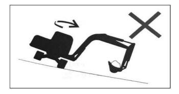
Do not operate the mini-excavator on a slope as far as possible.
