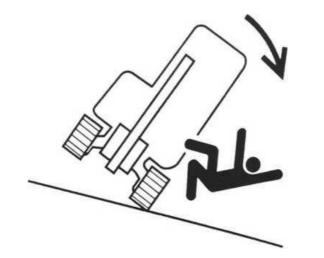
Do not change the direction of movement of the mini-excavator on a slope or cross slope. First return to the flat ground, and then choose another path.
