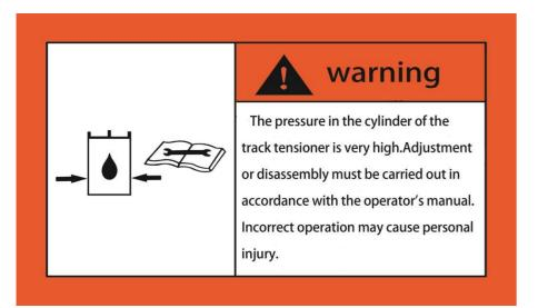
The pressure in the oil cylinder of the belt tensioner is very high. Adjustment or disassembly of the belt tensioner must be carried out in accordance with the operator's manual. Incorrect operation may cause personal injury.
