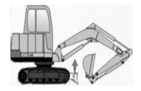
Avoid crossing obstacles as much as possible. If this is necessary, keep the bucket unit close to the ground, and walk it slowly. Do not cross obstacles that will tilt the mini-excavator by 10  $^{\circ}$  or more.
