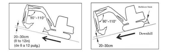
When climbing, keep the driver's seat facing the hillside. When going downhill, keep the driver's seat facing downhill. In both cases, pay attention to the ground state in front of the mini-excavator at the time of walking.
