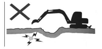
Do not work in the environment with collapse or rockfall hazards, and the corresponding protective measures should be taken.
