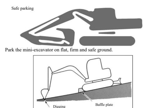
If it is necessary to park or tilt the mini-excavator on a slope, park the mini-excavator firmly and prevent the mini-excavator from moving. When parking on the street, grids, warning signs, lights, etc. shall be used to make the mini-excavator easy to see even at night to avoid collision with other vehicles.
