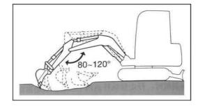
1. When excavating with stick and bucket, the excavation depth should be shallow and the excavation stroke should be long. The digging force is maximum when the angle between the swing arm and the bucket rod is 80 ° to 120 °. This angle should be used for effective excavation.
