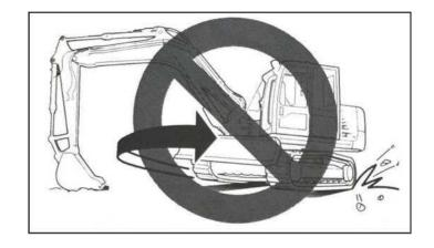
Do not use the bucket operation device to rotate the frame when raising it in front of the mini-excavator (there is no rotation on the mini-excavator). Otherwise, the load will be concentrated on the caterpillar band, and the single point is to twist the track, resulting in rapid damage and falling off of the caterpillar band.
