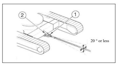
Serious injury or death may result from improper operation, use of wrong cables or improper inspection when towing the mini-excavator.
