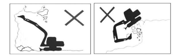
Do not work in the environment with collapse or rockfall hazards, and take corresponding protective measures.
