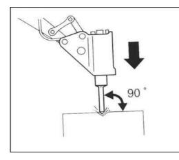
In order to avoid hitting the air, during crushing, the hammer head shall be properly aligned with the object to be crushed.
