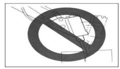
Do not pry the working surface with a hammer, and do not pry the working surface when it is broken; Do not move the hammer head when breaking.
