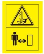
9. Hydraulic tank sign: this sign is located on the housing at the hydraulic oil tank.
