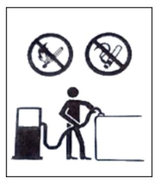
Do not smoke or have open flames when operation the mini-excavator with fuel or fuel systems. Do not carry fire sources, inflammable and explosive articles.
