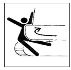
Do not place your hands, feet or other body parts in the middle of the caterpillar band of the mini-excavator. When the mini-excavator is started, it is strictly prohibited to stand other personnel within the operation radius and stack objects that hinder the operation of the mini-excavator. Avoid bumping and crushing damage.
