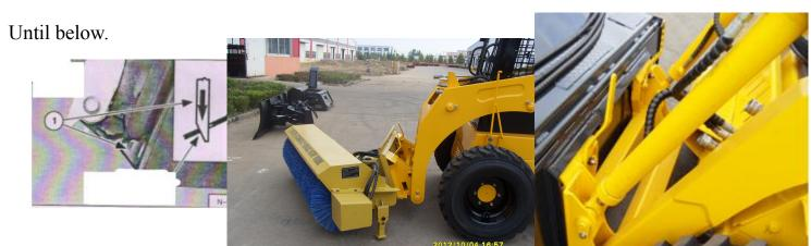
Tilt the quick-change rack backwards until the device slightly leaves the ground. Press and hold the wedge-shaped lock pin of the quick-change rack to switch downwards until the wedge-shaped lock pin completely penetrates the mounting bracket hole!
