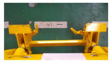
Drive the loader forward until the upper edge of the quick-change rack is completely on the upper flange of the quick-change device
