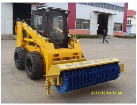
5. It is possible to adjust the left and right angle of the oblique cleaning machine to the rightmost deflection operation.
