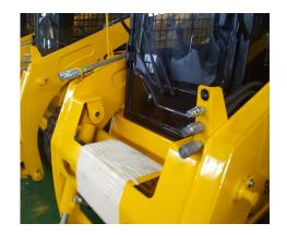
Note: Ensure that the quick connector is fully engaged. If the quick connector cannot be fully engaged, please check whether the size and type of the connector are the same. Before making connections, thoroughly clean the quick connectors. Dust can quickly damage the system.
