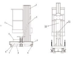
Guardrail 2. Aluminum mast 3. Oblique support rod
