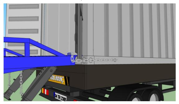
Put down the legs and turn the leg handle until legs slightly touch the ground. If the ground is not even, put some wood under the leg not touch ground.
