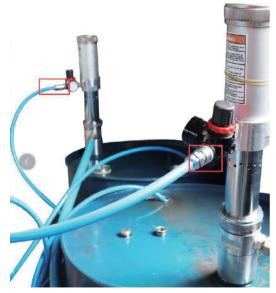
Connect air hose to compressor(above 32cfm ,116 psi )
