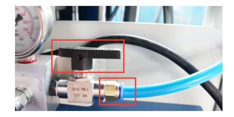
Return hose another side will connect to the small port of the drum(a side to a drum b side to b drum )
