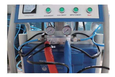
Connect the return hose to machine (at winter cold day ,better to connect return hose and open it to recycle material for in advance heating ,when you finish recycling,turn off the two valves from a and b side )
