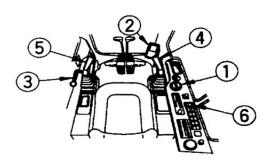
$\hfill\Box$  Put the safety lock lever in the release position and lift the bucket from the ground.
