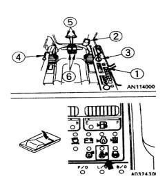
☐ Fold back the working device and lift it off the ground40cm~50cm₀
