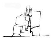
When operating on a slope, the excavator should avoid turning to prevent rollover or side sliding accidents.
