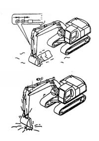
reducing the service life of the machine. To prevent this from happening, always keep a small safety distance when operating the □□ Patayyeindeotpærratitoion the hydraulic cylinder to the end of its stroke: During operation, if the hydraulic cylinder is operated to the end of its stroke, the force will be applied the internal stop of the cylinder, thereby reducing the service life of the machine. To this from prevent happening, always keep a small safety distance when operating the cylinder...
