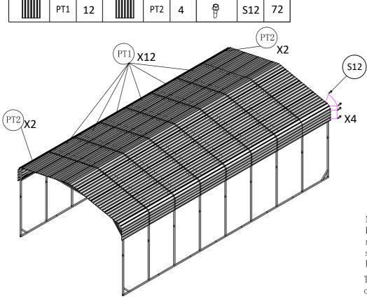
NOTED: Both end of Panels PT1 have holes, Please noted the short holes space are connect with Panels PT2.
